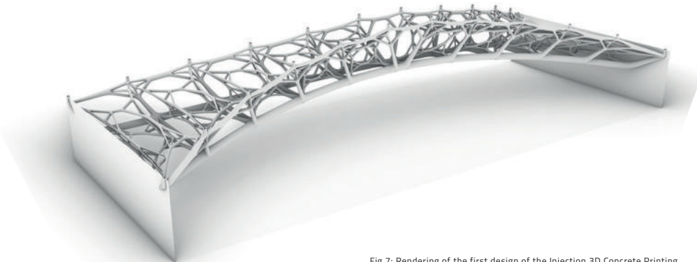
Fig 7: Rendering of the first design of the Injection 3D Concrete Printing demonstrator (bridge with 10m length) based on the principles of graphic statics. Designed by P. D'Acunto (TU Munich) and O. Ohlebrock (ETH Zürich) [5]
