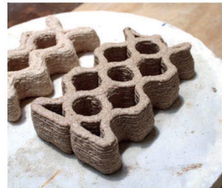
Fig 16: 17th mix - oval squared shaped undulation Observations: material overaccumulation on the corners
