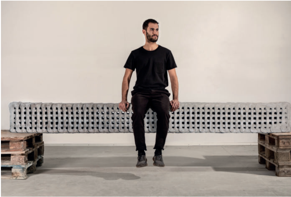
Fig. 4A: prototype of GridBeam, a three-metre porous slab with a grid pattern and a woven layered extrusion;
