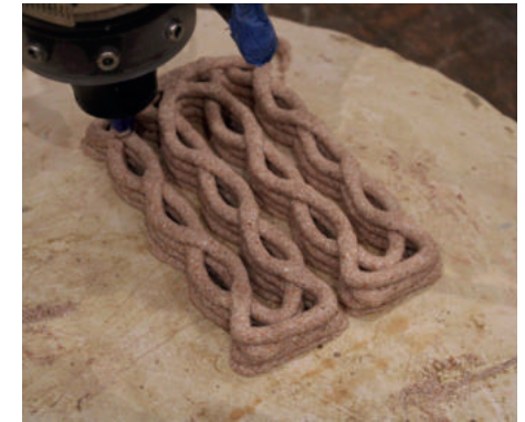
Fig 15: 10th mix - increased layerheight and cross supports Observations: geometry provides reinforcement, excessive accumulation of material, optimal viscosity
