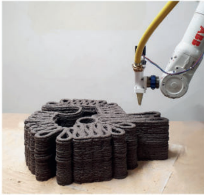
Fig. 4: Robotic 3D printing of the demonstrator components, and subsequent point-cloud tracking of the geometric deformations due to evaporative cooling
