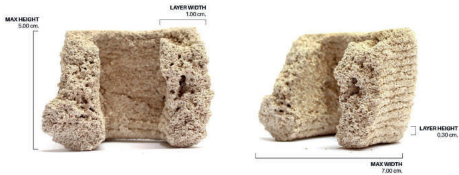
Fig 6/7: 3D Printed eggshell section detail These are some of the selected tests that show the characterization of the behavior under certain geometries and the modifications on the mix through time:
