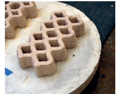
Fig 17: 20th mix - more organic undulation, allowing more stability Observations: geometry allows more continues printing
