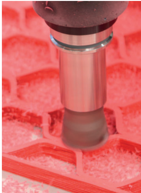
Fig. 7B: Robotic milling of the core surfaces
