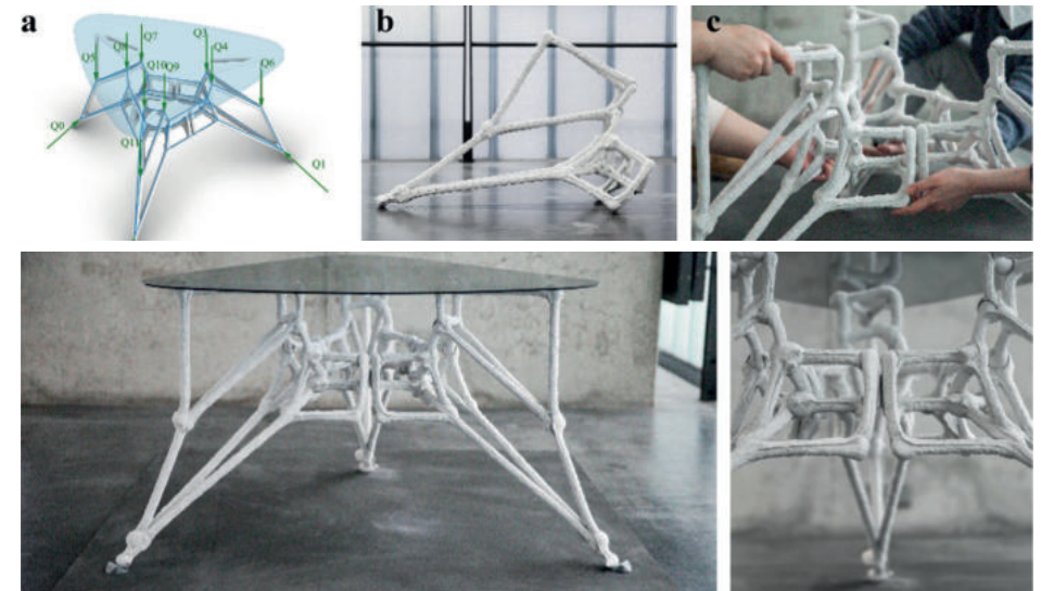
Fig 5: (a) Form diagram of the table; (b) One leg of the table as a segment; (c) The process of assembling the printed segments into a whole table (top); the assembled lightweight concrete table demonstrator (bottom) [6]
