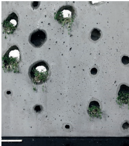
Fig 10: Schematic Suspension in Concrete (SiC) process (top) and 30x30 cm 2 application (bottom) [4]
