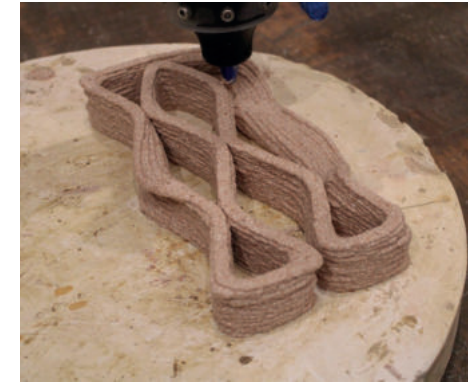
Fig 13: 8th mix - geometry test Print reaching geometric limit
