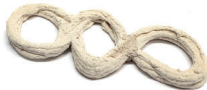
Fig 9: Second mix - 0.1% less xanthan gum, 4.2% less water content Observations: bad stability, mix too liquid
