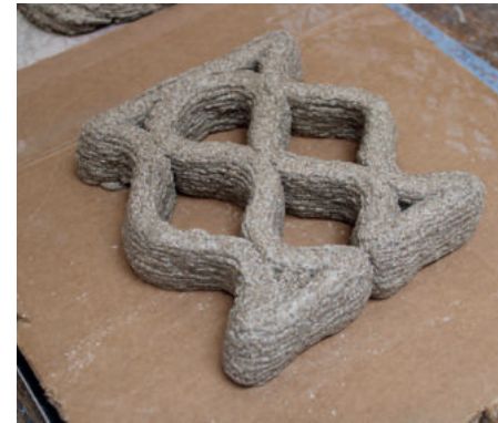
Fig 14: 7th mix - mid-scaled model Observations: appropriate scale, material without enough structure
