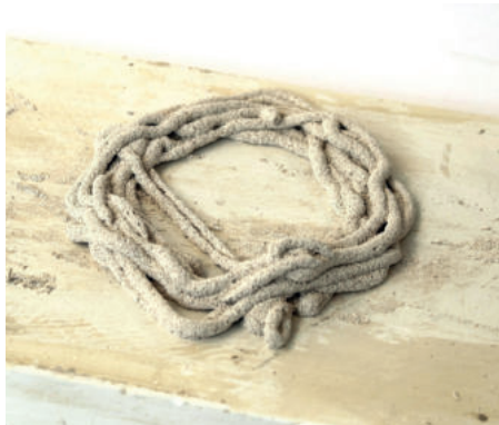
Fig 8: Initial mix Observations: required infill
