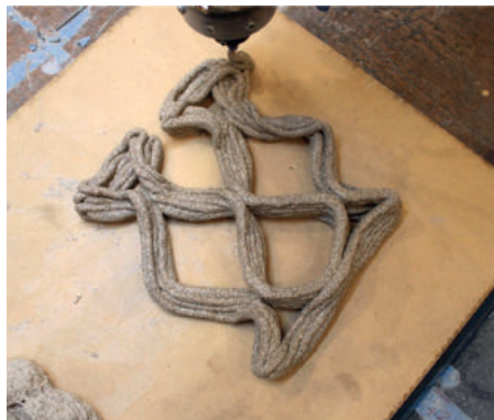
Fig 11: 4th mix - scaled up model, 0.1% more xanthan gum Observations: limited rigidity, enlarged scale leads and geometry provides insufficient support and inadequate contact between individual layers
