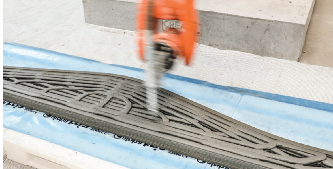
Fig 3: Robotic 3DCP fabrications in the CREATE Lab at the University of Southern Denmark.
