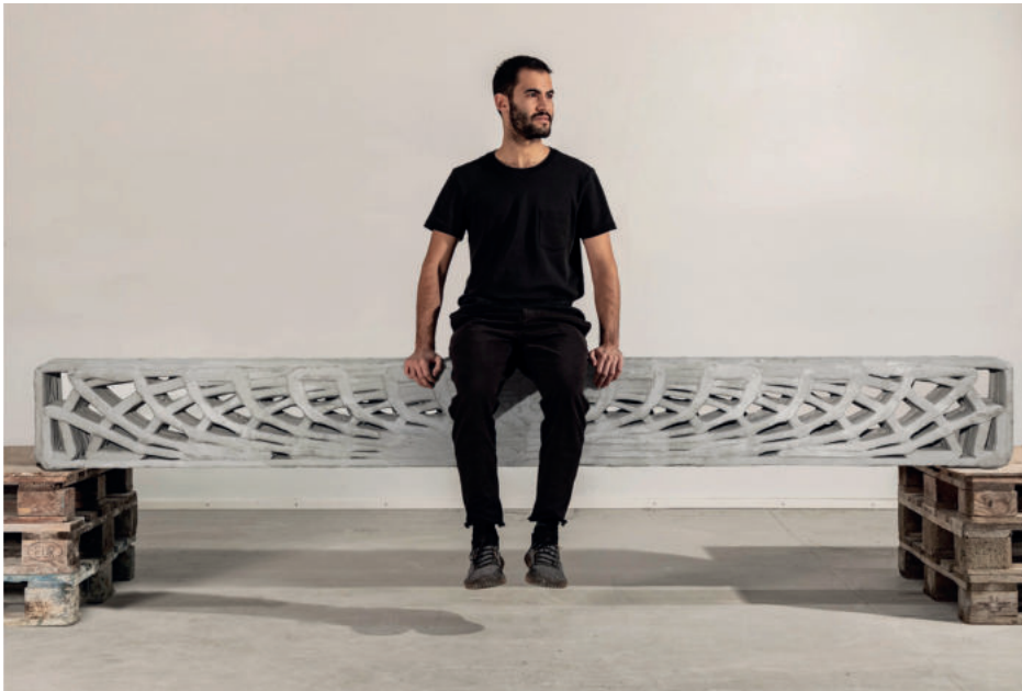
Fig 4B: outlook of 3DLightBeam, a 3DCP lightweight beam that integrates FEA-generated PSL as a design driver.
