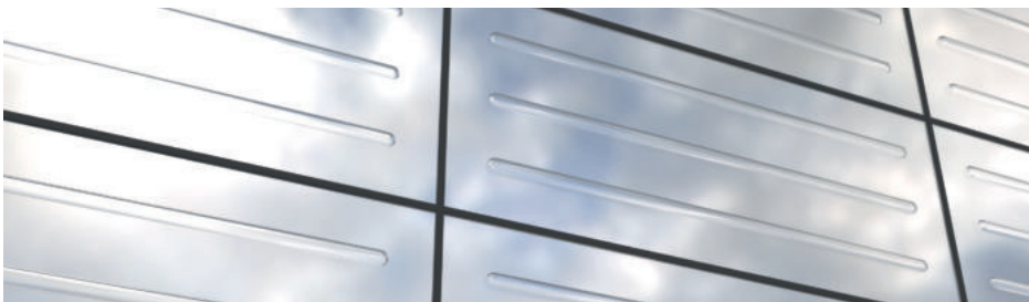
Fig. 3: Rendering of flatt glass with reinforced cross section due to AM ribs
