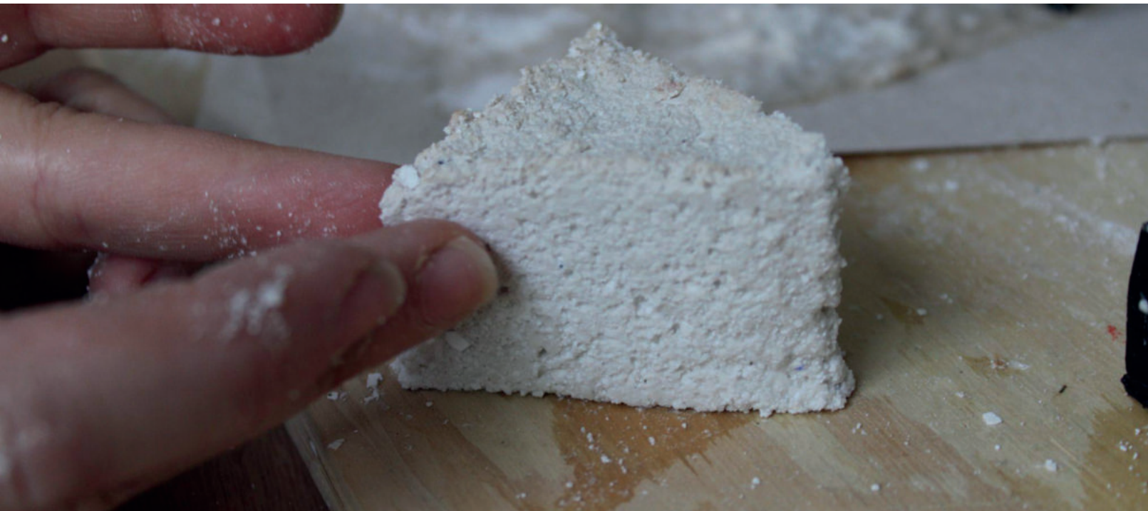
Fig 5: First prototypes based on a PLA 3D printed plastic formwork
